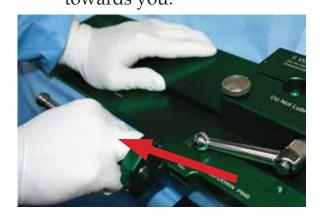
While holding the pin at the bottom, rotate it to the upright and locked position.
