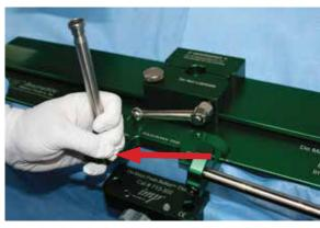
To lower the pin, grab the pin at the bottom and pull the pin creating a gap at the pin base.
