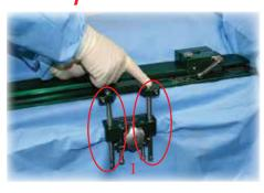
1 ~ Confirm the sliding pins are pushed completely down and fully seated in the clamp.
