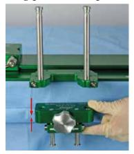
3. Tighten the Clamp Knob by turning it clockwise.
