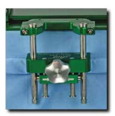
4. Seat the sliding pins in the Clamp holes.
