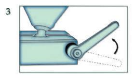
Rotate, counter-clockwise, while holding in the pulled-out position
