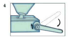
Release, at desired position snapping into gear, and
