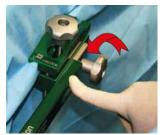
With the appropriate side leg showing on the extension, slide the cut out of the extension over the clamp's metal bar and side knob until it stops
