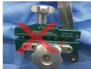
Vertical Bar is not vertical and only touches clamp's top jaw slot edge.
