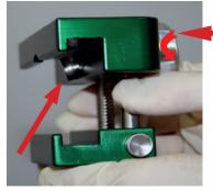
1. Loosen the Clamp Knob all the way by turning it counter clockwise. The leading "cap" should be flush to the upper jaw.
