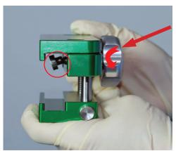
1. Loosen the Clamp Knob all the way by turning it counter clockwise.
