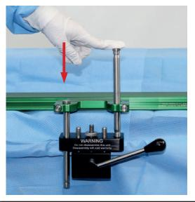
7. Slide and seat pins into holes of the clamp.
